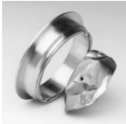
In relief valve applications, install a nonshattering rupture disc (left) upstream of the valve. A disc that fragments when it ruptures (below) is acceptable if no relief valve is present.
