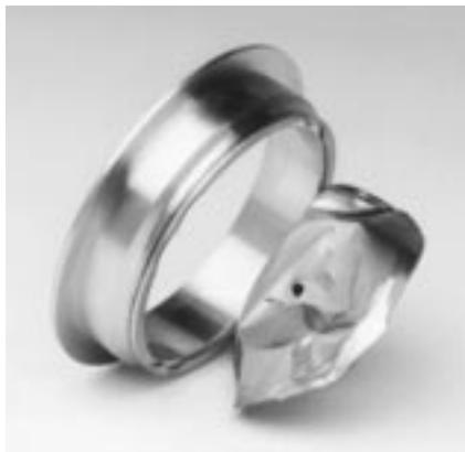
In relief valve applications, install a nonshattering rupture disc (left) upstream of the valve. A disc that fragments when it ruptures (below) is acceptable if no relief valve is present.
