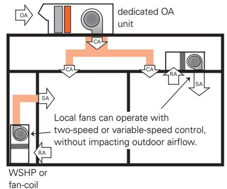
For this example, two-speed fan control (constant fan speed when heating) reduced HVAC energy use by about 25 percent, while variable-speed fan control (capable of variable fan speed when heating) reduced HVAC energy use by about 30 percent.
