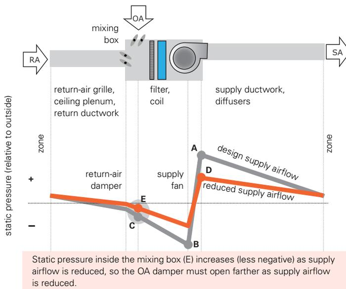
This method is not perfectly accurate over the entire range of airflows, since damper performance is nonlinear. And it does not account for outside influences like wind or stack effect. Therefore, it does result in some over-ventilation in the middle of the fan speed range, but much less over-ventilation than if a fixed-position damper were used (see inset).
