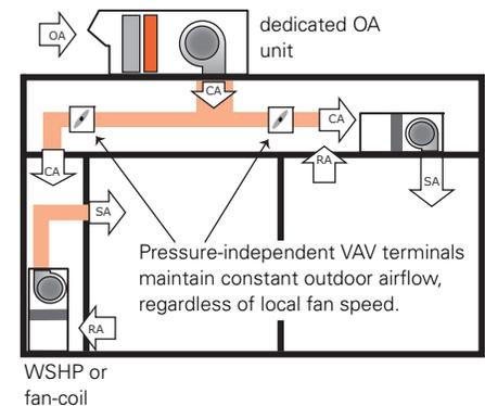
**Figure 9. Conditioned OA delivered directly to each zone**
