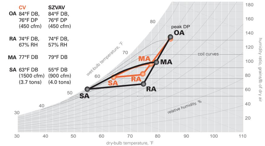
**Design air distribution system to accommodate variable airflow.** Use diffusers that will provide proper air distribution at reduced airflows. Diffusers that are appropriate for conventional VAV systems are probably best suited.
