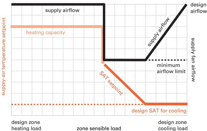
**Figure 4. Example SZVAV control with two-speed fan**
