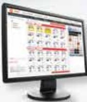
**System controls** provide a higher level of management for multiple-VRF systems, as might be found in a multi-floor building. System controls provide more-advanced scheduling, operation and alarm history management; they can be accessed remotely for monitoring via an Internet connection.
