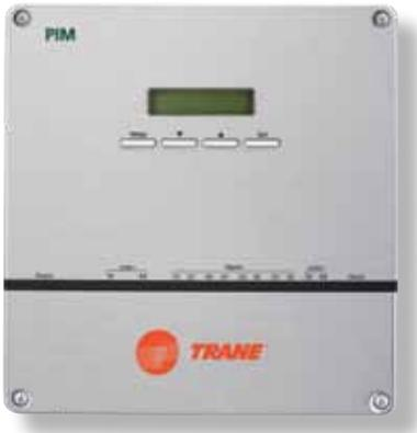
**System controls** provide a higher level of management for multiple VRF systems, as might be found in a multi-floor building. System controls provide more-advanced scheduling, operation and alarm history management; they can be accessed remotely for monitoring via an Internet connection.
