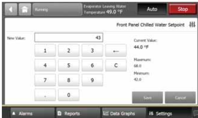
Figure 55. Changed chilled water setpoint screen
