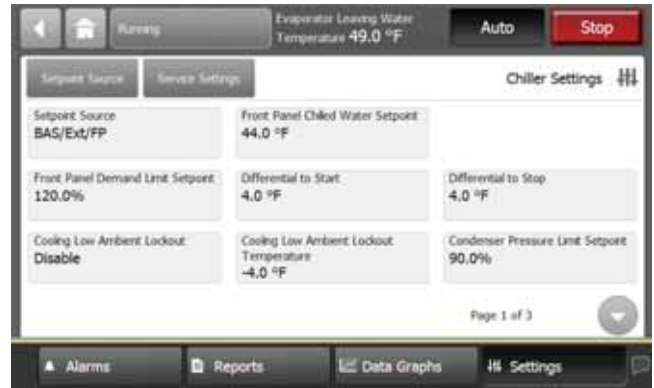
Figure 53. Equipment setting screen (Chiller setting shown)
