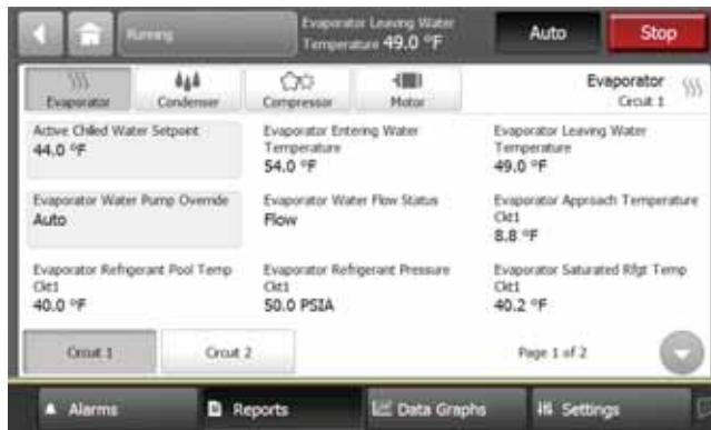
Figure 47. Report evaporator screen
