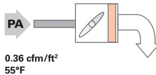
**VAV terminal with 40% minimum airflow setting**
