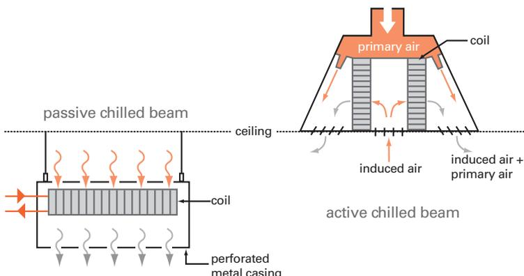
Figure 2. Examples of active chilled beams
